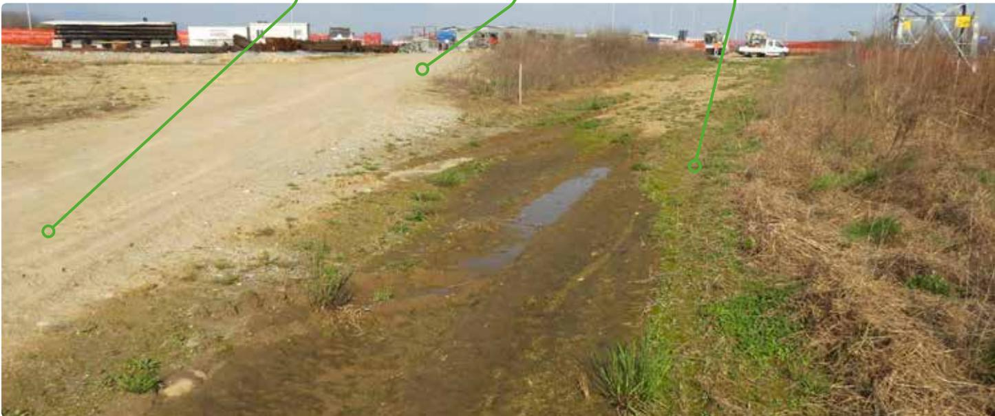
Tests 1 and 2 were made on the same road but with different aggregates and different application methods. Both treated areas were very compacted.
