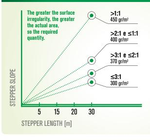
The quantity of **HYDROMAT®** is determined by the gradient, the slope condition, the soil texture and weather conditions.
